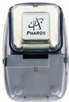
A digital camera add-on device for geotagging photos.
