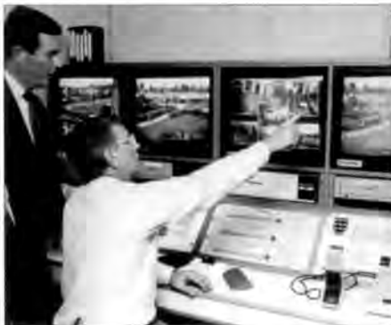
The new CCTV system from Neurodynamics can assist a sole operator to watch several locations from miles away and simultaneously. An alarm alerts the watcher of suspicious movements.
