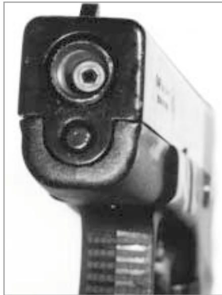
THE PLATE: Semi-auto blank firing pistols must have some kind of restrictor plate threaded inside the barrel.
