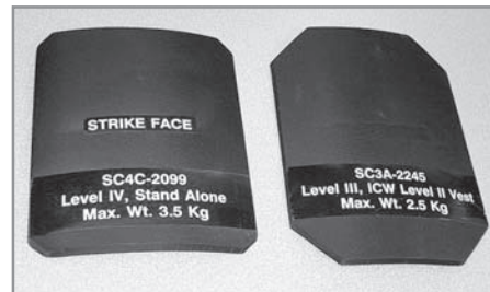
Level III and Level IV ceramic plates
