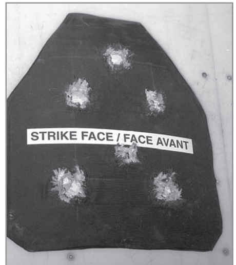
Ceramic plate shot with 6 rounds of 7.62x51 NATO ball
