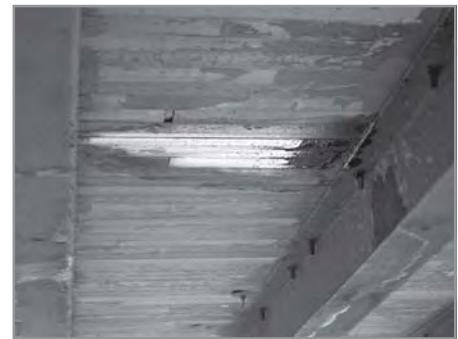
Picture 2: Underside of trailer leaking acid
